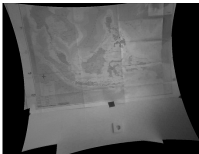
Fig. 15. Image captured from distance of 1 meter with 0^\circ of angle between cameras after being stitched
