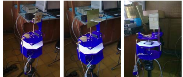
Fig. 8 The load test using patch antenna with dimensions of 61mm x 60mm and weight of 50grams (left), patch antenna with dimensions of 80mm x 80mm and weight of 100gram (center) and patch antenna with dimensions of 119mm x 75mm and weight of 100gram (right).
