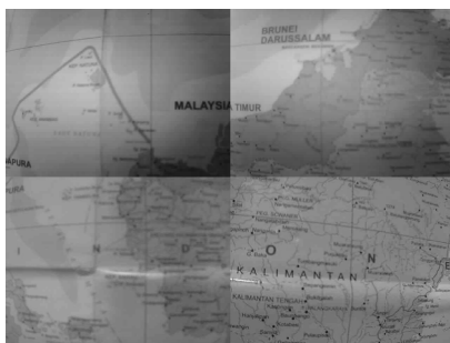
Fig. 17. Map with 1:4,750,000 scale captured with 4 cameras from distance of 14.7 cm and 30^\circ of angle between cameras.
