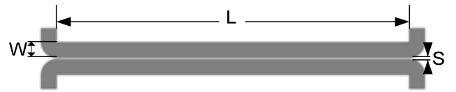
Fig. 3. The proposed design layout of directional coupler.
