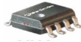
Fig. 16. An RF power amplifier VNA-23 [12]
